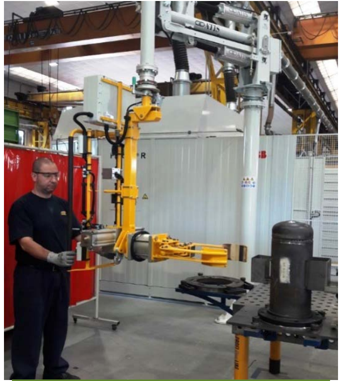
Operator Francesco Di Maria prepares for a lift with the Zero-Gravity Pneumatic Manipulator
